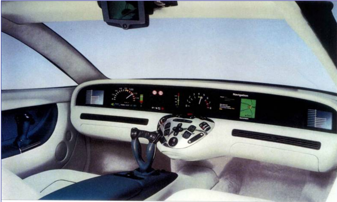
A revolutionary interior: Linked to drive-by-wire electronics, the central sidestick replaces steering wheel and pedals.
