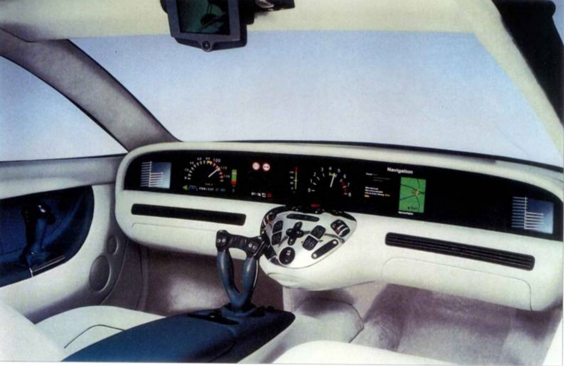
A revolutionary interior: Linked to drive-by-wire electronics, the central sidestick replaces steering wheel and pedals.
